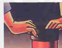
1. Push Sealing on end of pipe
