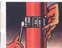
5. Screw both ends firmly, ensuring that both plates are parallel
