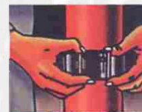
4. Lay collar around sealing
